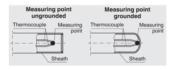
For temperature measurement in a solid body, the diameter of the bore into which the probe should be inserted, should be no more than 1 mm larger than the probe diameter.
