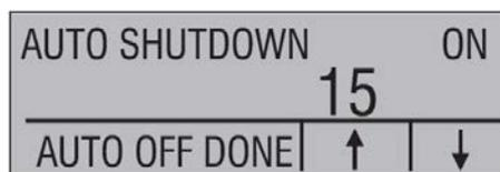
Use the "AUTO OFF DONE" option to set the parameters and return home. The auto shut-off time is reset whenever a key is pressed.
